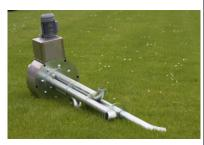
Type R works similarly to ordinary steam soot blower, but without the consequences of eroding the boiler tubes when using valuable steam that should be used for production purposes rather than cleaning.
